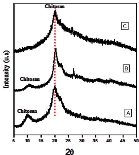
**Fig.1** X-ray diffraction. A) powder chitosan; B) chitosan beads without crosslinking; C) beads crosslinked with 2.5% glutaraldehyde
