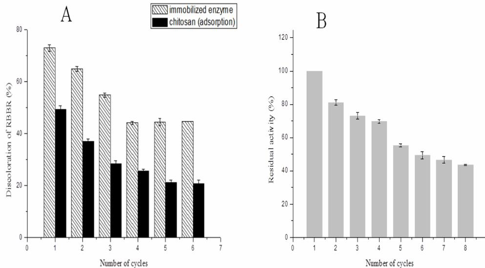
**Fig.6** A) Removal of 50 mg L<sup>-1</sup> Remazol Brilliant Blue R with repeated applications of immobilized turnip peroxidase; B) Operating stability of the immobilized turnip peroxidase. Data are the average of three replicates
