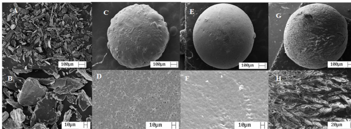
**Fig.2** Scanning electron microscope (SEM) images. A) chitosan powder (100 μm) ; B) chitosan powder (10 μm); C) beads without cross-linking (100 μm); D) beads without cross-linking (10 μm); E) chitosan beads crosslinked with 2.5% glutaraldehyde (100 μm); F) beads cross-linking with 2.5% glutaraldehyde (10 μm); G) chitosan beads after immobilization of peroxidase (100 μm); H) chitosan beads after immobilization of peroxidase (20 μm)
