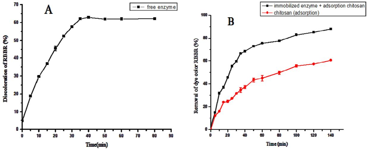
**Fig.5** Reaction progress on the discoloration of Remazol Brilliant Blue R. A) free turnip peroxidase; B) immobilized turnip peroxidase and adsorption on chitosan. Data are the average of three replicates
